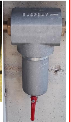
STEEL FILTERS (50 micron) About 1000 l sampled in drinking water
