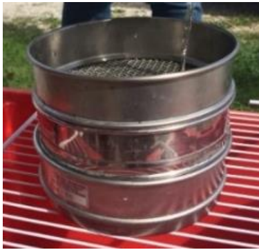
PUMPING AND SEIVING (50 micron) About 1000 l sampled in drinking water
