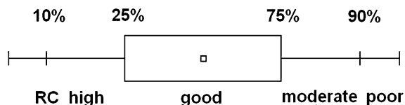
Fig. 2 Classification criteria based on the statistical distribution of geometric mean values of the water quality metrics in Lake Vörtsjärv for the period studied. It was supposed that half of the measurements (25th–75th percentile) should indicate the “good” quality class mostly identified by previous studies. Reference conditions were defined as the median of the “high” class values
