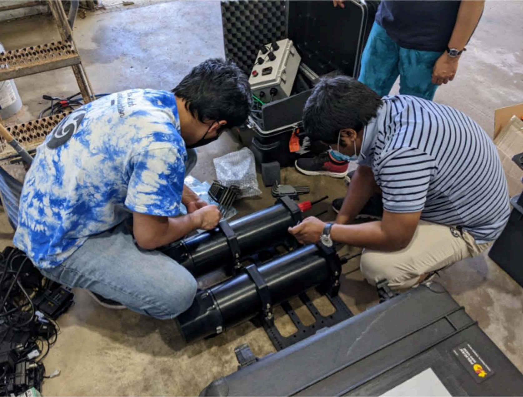
Researchers work on an AUTOHOLO device, which uses holographic technology to image and detect harmful algal blooms. Photo by Aditya Nayak, Florida Atlantic University.
