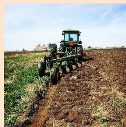
Pic. 1: Tractor with chisel plows, a good way to implement a reduced tillage with depth of around 15 cm
