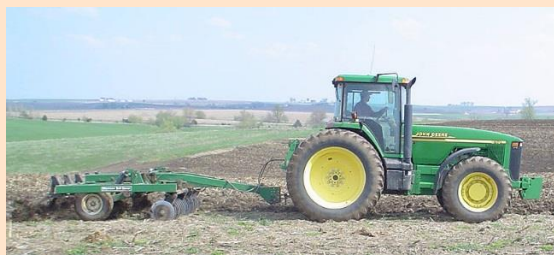
Pic. 1: Tractor with chisel plows, a good way to implement a reduced tillage with depth of around 15 cm
